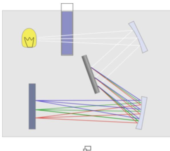
Diagram of a single-beam UV/vis spectrophotometer.
